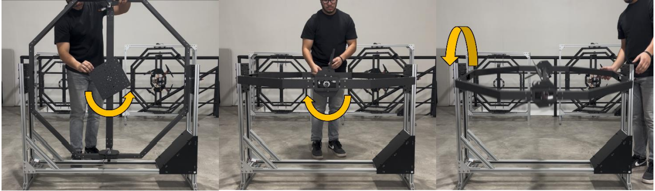
Figure 13. Movement verification of Yaw, Roll and Pitch movements (from left to right).
