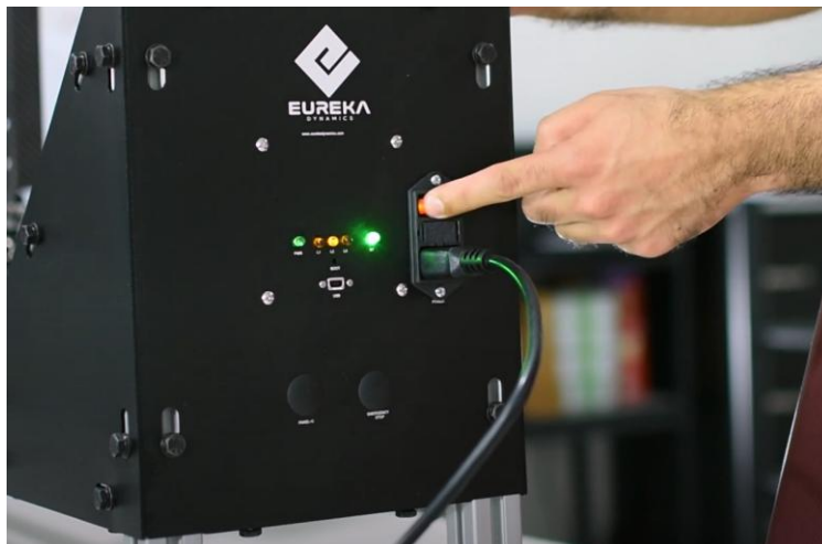
Figure 19. Turning-on the FFT GYRO.
