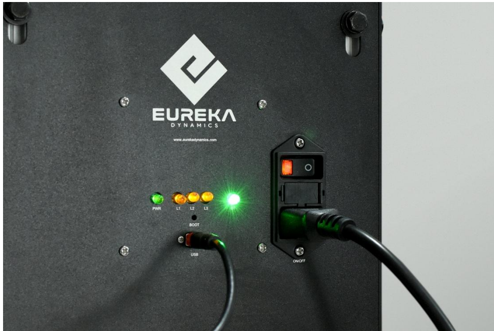
Figure 14. Mini-USB cable connected to the FFT GYRO's front panel.
